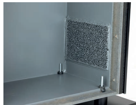
The ceramic foam plate in the Classic 35 is positioned in front of the bassreflex vent as a damping element and helps to minimize flow noise
