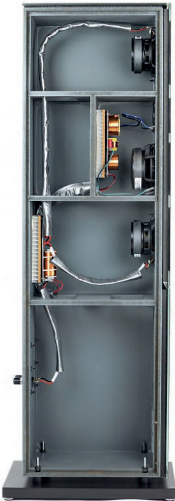
The two woofers use a common vented volume. A sealed chamber provides ideal operating conditions for the 150 mm midrange driver
