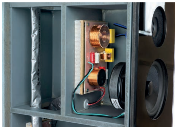
Honeycomb-Sandwich boards are used as decoupling carriers for the crossovers. The midrange's flat phase plug optimizes the thermal behaviour of the driver
