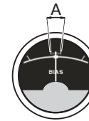
Diagram 5 Bias meter during working Note: When working normally, the pointer should stay within the A zone, still, it would move for the voltage fluctuation.
